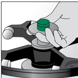
◀ Push center button to remove rotor
