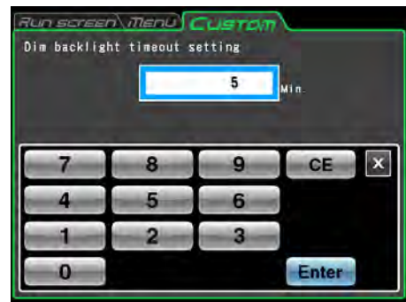
Fig. 3-4-5 (4c) Screen for setting the time period after which the backlight will be dimmed
