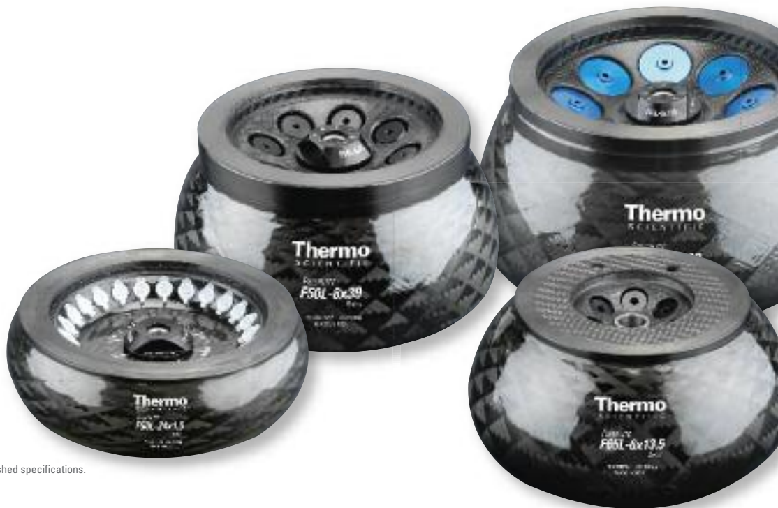
Figure 10: Fiberlite ultraspeed rotors (counterclockwise from top right): F40L-8x100 (40,000 rpm; 213,200 xg); F50L-8x39 (50,000 rpm; 266,200 xg); F50L-24x1.5 (50,000 rpm; 280,000 xg); F65L-6x13.5 (65,000 rpm; 324,100 xg).
