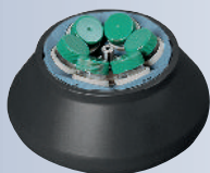
Angle rotor, Cat. No. 01620A 6-place, n = 9,000 min -1 , max. RCF 9,418. illustrated with adapter set 01646
