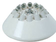
Angle rotor, Cat. No. 01615 12-place, n = 12,000 min -1 , max. RCF 16,582
