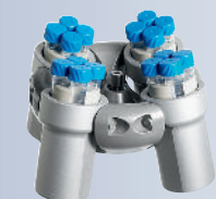
Swing-out rotor 01324, 4-place, illustrated with suspension 01398 and adapter 01483 n= 4,500 min -1 , max. RCF 3,260
