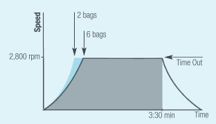
**Figure 1:** In a typical first centrifugation step, a two-bag rotor load attains set speed faster than a six-bag load. Since both loads will time out at the set time of 3:30 minutes, different g-forces are achieved during the run. By using the ACE integrator function, the time for 2 bags would be changed to 3:00 minutes to obtain the same overall g-force for both loads.
