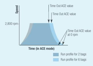
**Figure 2:** With an ACE value and speed set at the start of a run, times were adjusted to achieve the same overall g-force regardless of the rotor load.
