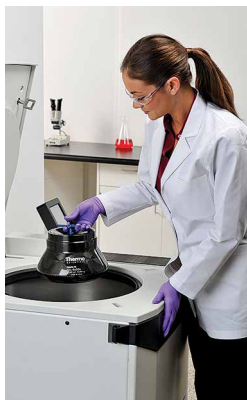
1. Place rotor into the centrifuge chamber
