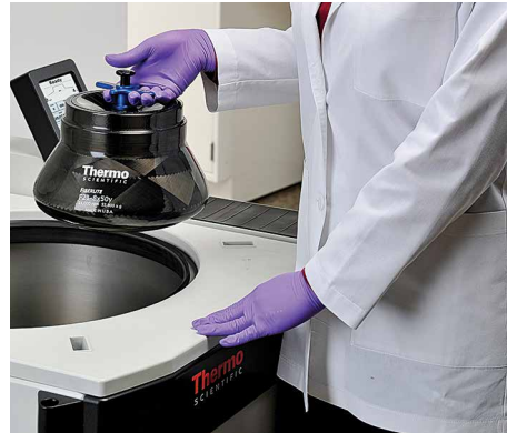
Lightweight rotors with speed handles
