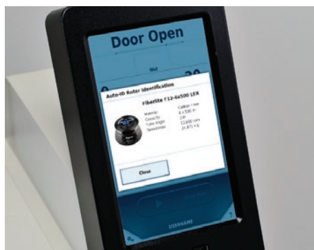
Figure 8. Auto-ID instant rotor identification. Improves safety, saves times, and protects the integrity of your samples.
