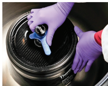
Figure 9. Speed handle on rotor lids. Makes tightening the lid safer while also simplifying lid removal.
