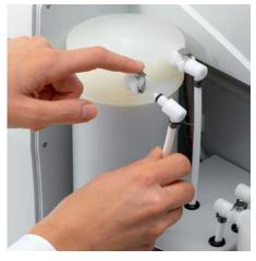
**One, two, three...** ... rapid cartridge change due to quickconnects.
