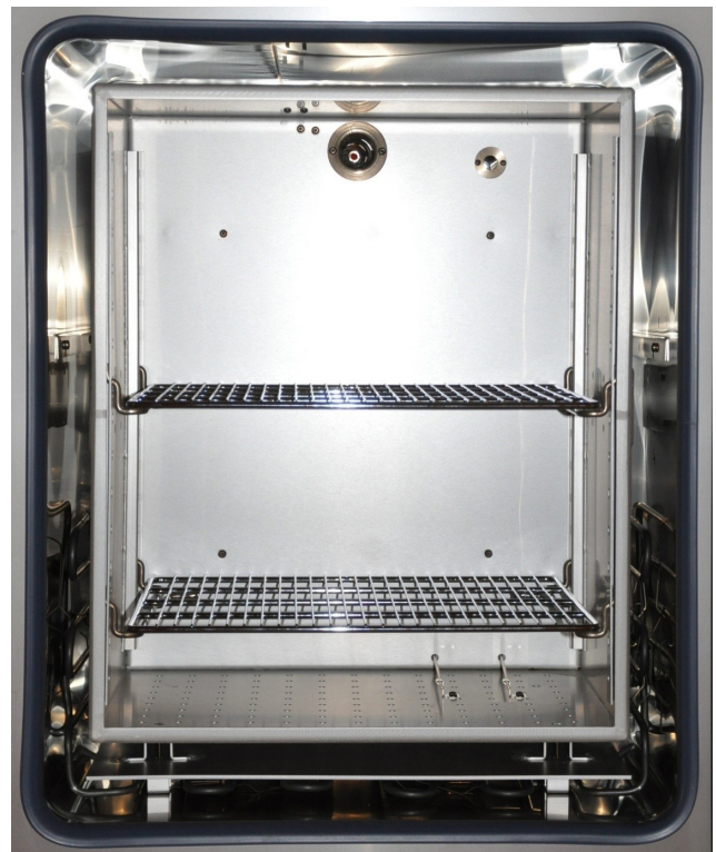
Interior of OGH TK 100 with aluminum ISO box
