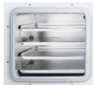
Vacuum chamber with two additional shelves
