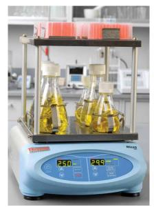
Figure 1. Thermo Scientific MaxQ 2000 shaker with 11" x 13" dual tiered platform
