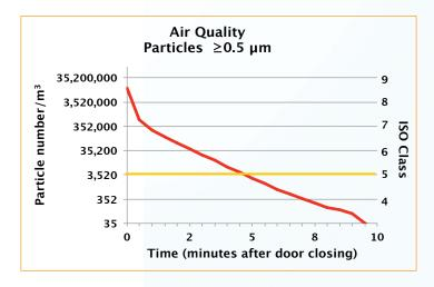
Our unique HEPA air filtration design reaches ISO Class 5 cleanroom air quality and recovers to that quality of air after a door closing within 5 minutes as tested in accordance with ISO 14644-1 and ISO 14644-3.
