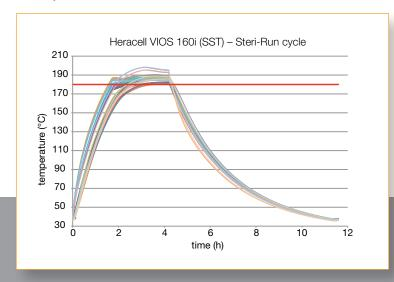
The U.S. and E.U. Pharmacopeias no longer recommend a given temperature and time for sterilization. Instead, they require proof of performance. To meet requirements of a 12 log SAL, a 6 log reduction of biological indicator endospores must be demonstrated in half the time.
