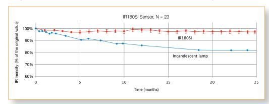
A traditional IR sensor contains an incandescent bulb that puts out less light as it ages, resulting in sensor drift. The IR180Si eliminates this problem. Our silicon MEMS emitter is designed to retain intensity over time, lasting up to 50% longer than ordinary IR sensors.
