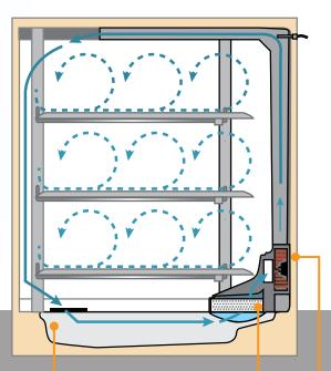
Incoming air first travels over a direct heated water reservoir resulting in 50% faster humidity recovery than with a standard water pan design.\*\* The in-line HEPA filter cleans the airstream of microbes and particles protecting cultures from contamination.
