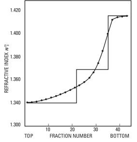
Fig. 4. Shape of the gradient after centrifugation. Refractive index.  $n_{\rm D}^{\rm 25}$  determined using a Bausch & Lomb ABBE-3L refractometer. The shape of the discontinuous gradient prior to centrifugation is shown by the dotted line.
